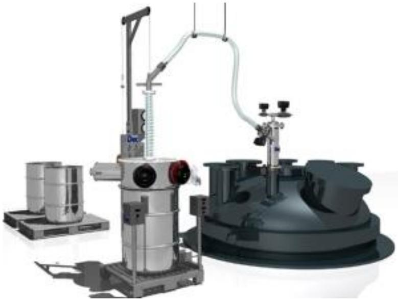
*DCS Drum Discharging Station combined with PTS for pneumatic reactor feeding*
