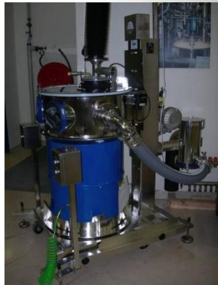
*Right: DCS Liquid System for drum discharging with corrosive and toxic liquids*
