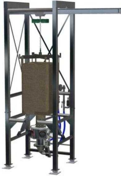
Optionnally, both systems filling and discharging are available with load cell features to provide accurate dosing, sampling features and for inert operation.
