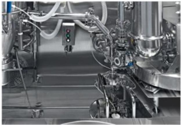
Inside view of micronizing isolator for safe and contained operation
