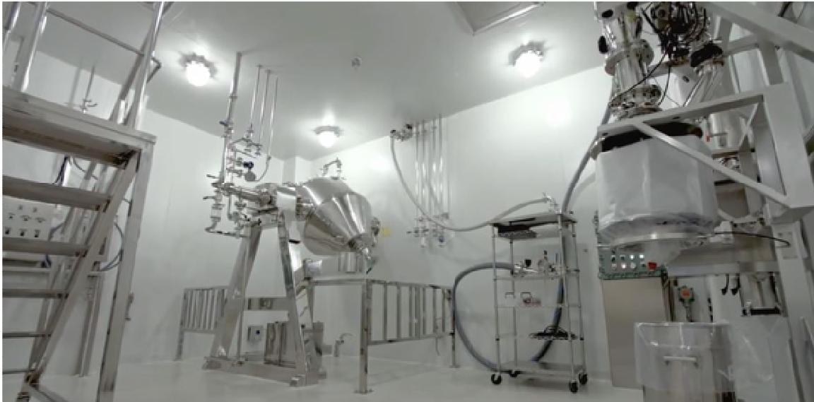
Left: Rotating filter Dryer with Safe Dock-Valve, right: Continuous Liner System with PTS and DosiValve
