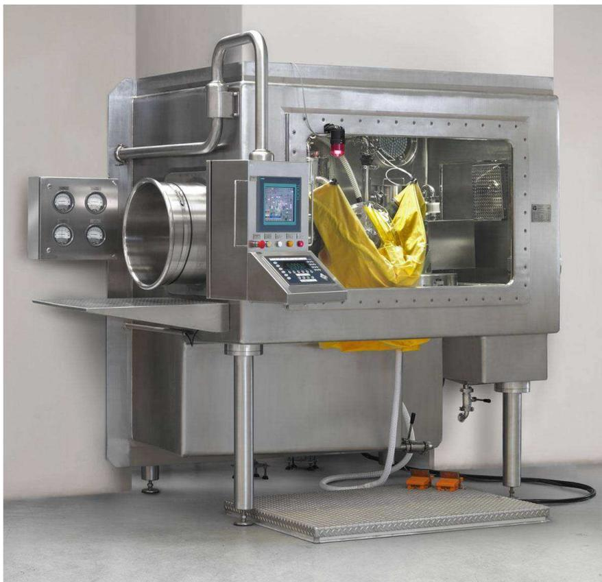
The latest generation of MC Jetmill® systems has been developed with Computational Fluid Dynamics (CFD) analysis, combining high innovation with enhanced performance: The CFD improved geometry of the grinding chamber enable exceptionally narrow particle size distribution (PSD) around 1 micron (Gaussian curve), even with very sticky, fine and adhesive powders. The newly ring integrated nozzles represent a
