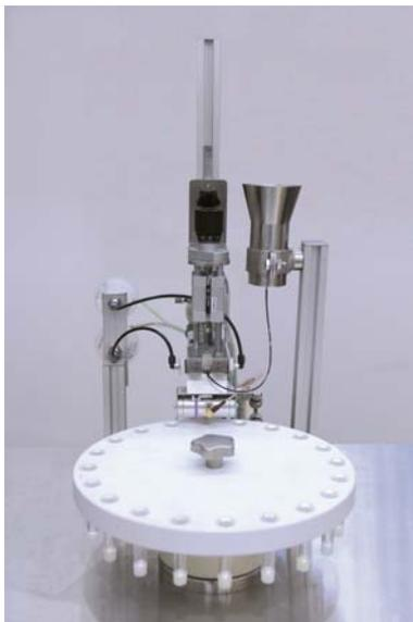
The Dec Group Exposition stand at Booth 1304 at the Orlando County Convention Center will feature live demonstrations of the MicroPTS, showing its abilities to handle volumetric dosing of powders down to 0.5 µg, which can be adjusted during process. The MicroPTS uses vacuum to fill its variable volume calibrated chamber and the emptying is done mechanically and/or by gravity and/or with pressure. PTS technology
