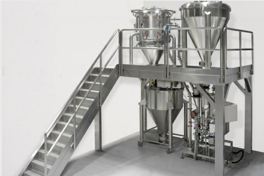
MC DecJet® 300 production plant (5 - 200 kg/h production capacity)
