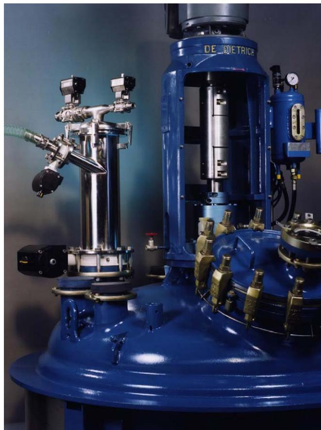
Fig. 9. Powder Transfer System (PTS).
