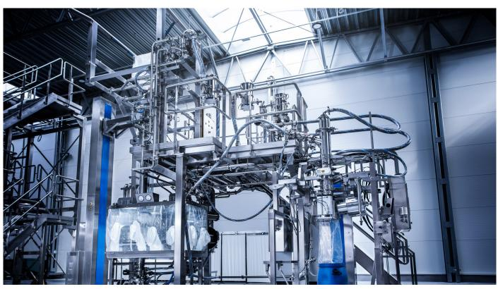
Pack-off suite integrating big bag gravity discharge, sieving in isolator, PTS transfer into pack-off unit for drums or big bags (interchangeable version)
