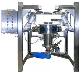
Loss-in-weight solution: Dosing by subtraction from big bags with DCS® Docl
