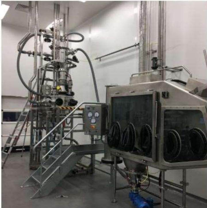
Drum/bag dispensing into FIBCs, Isocharge and DCS Big Bag Filling Station with PTS and DosiValve®
