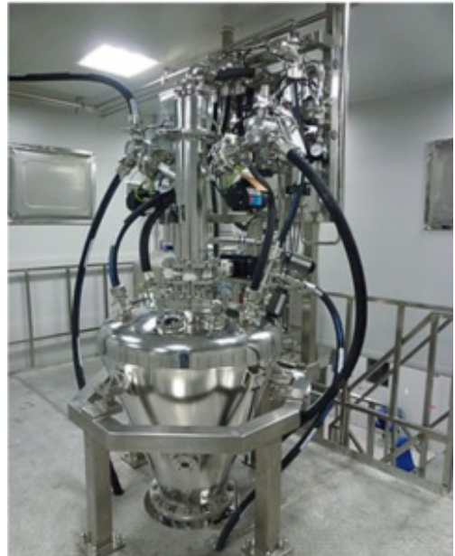
PTS Batchmixer®: New mixing technology without rotating or moving parts
