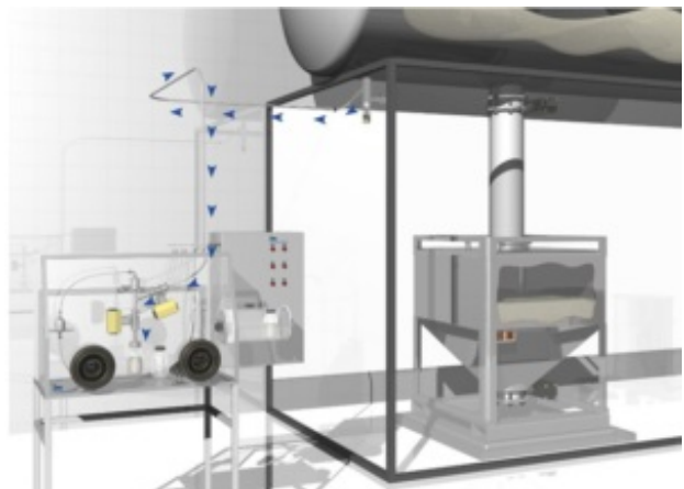
Dec High Containment Pack-off station for dryer discharge including upstream milling process
