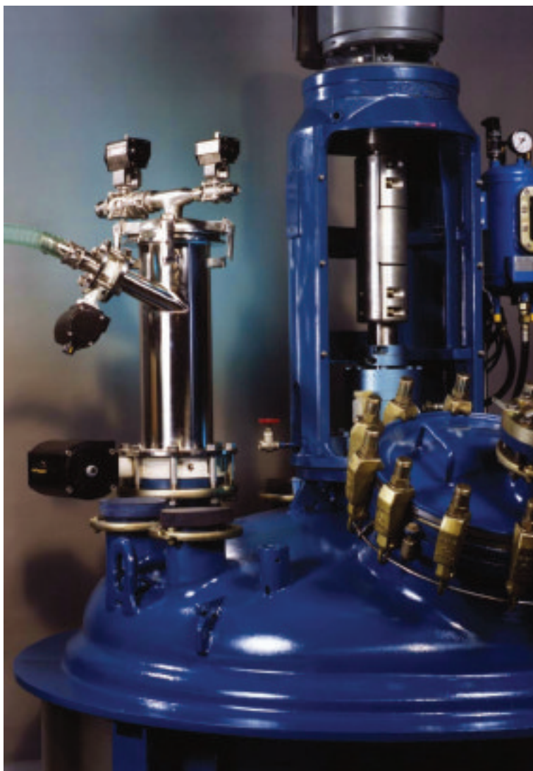
Figure 2: PTS installed on the nozzle of a reaction vessel
