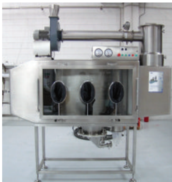
Figure 3: Isocharge Station for small and medium sized bags of powder
