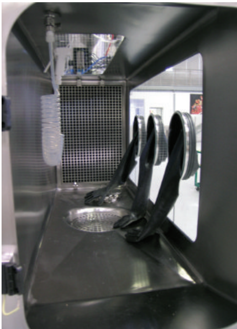
Figure 4: Inside the main chamber – a hybrid of isolator and laminar flow booth
