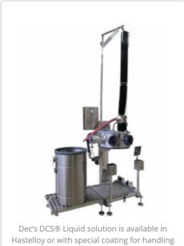
Hastelloy or with special coating for handling corrosive materials and can be fitted with castors for mobility.
