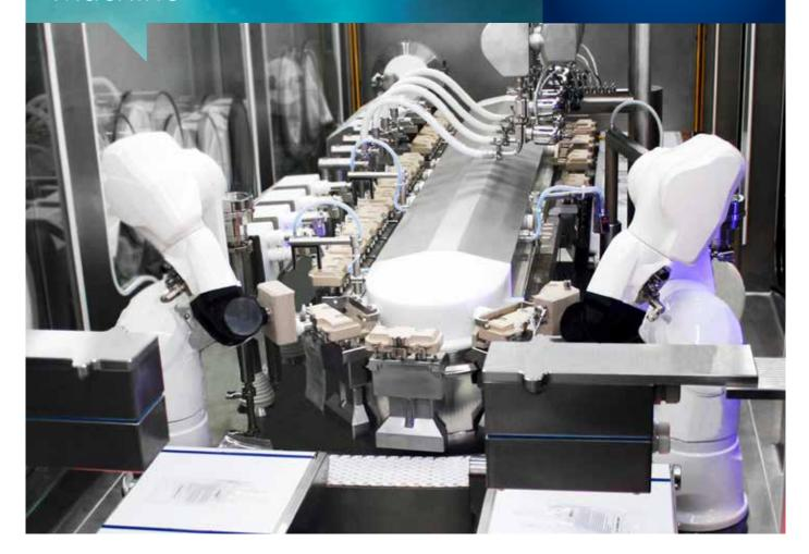
Automated aseptic filling and sealing machine for single chamber, dual chamber or triple chamber IV bags
