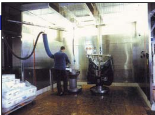
FIGURE 7. Containers may be equipped with flexible intermediate bulk containers (FIBC) fitted with docking devices that enable a receiver to be connected or disconnected in an almost airtight manner
