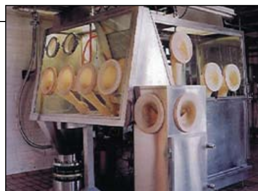
FIGURE 8. Glove boxes offer one of the only solutions to protect the operator, product and environment from a product with high toxicity
