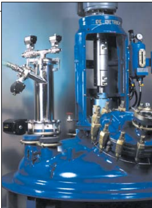
FIGURE 9. Specially designed powder transfer systems specifically address the safety risks related to transferring powders into solvents
