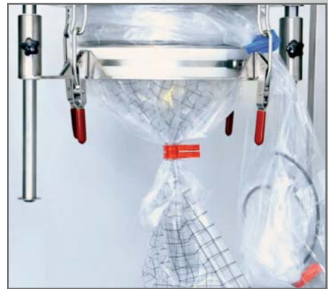
Abscission by cutting off the filled big bag underneath the ring with the help of a double clip.
