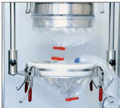
Release and lowering of the ring and abscission of the intermediate liner by cutting off between the two clips.
