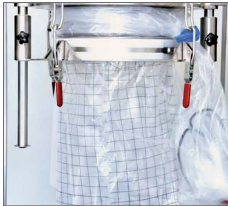
Lifting and clamping of the sealing ring to the filling tube. The system is now ready for product transfer.
